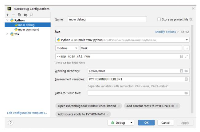
If the parameters are correct, then the Run dropdown menu will show green icons for run and debug. If the only choice under the Run menu is Edit Configuration, then one of the parameters is wrong, try again. Note: Py`Charm has a tendency to change the Working Directory field when other values are edited. Be sure it points to the repo root.
